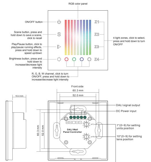
Rotary switches for setting start DALI address number (0-63), the number equals to tens position plus units position
