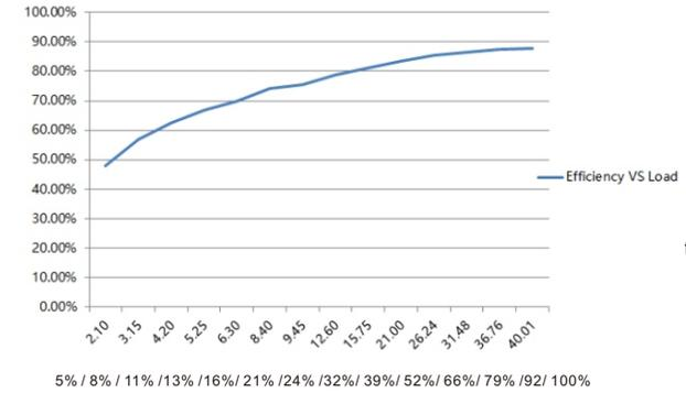
Note: Test data under 1050mA gear
