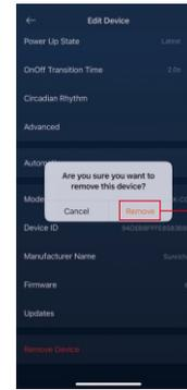
From your ZigBee controller or hub interface, choose to delete or reset the lighting device as instructed. The connected light blinks 3 times to indicate successful reset.
