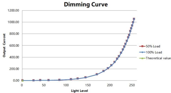
Note: Test data under 1050mA gear
