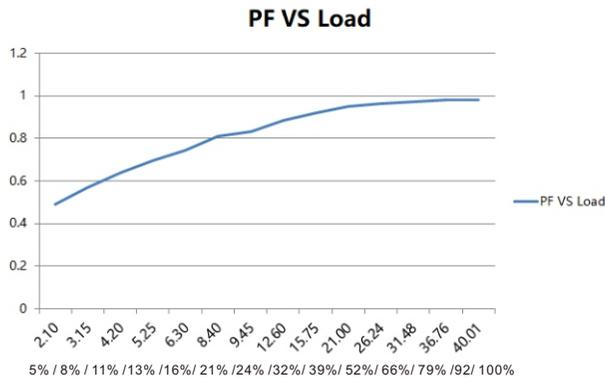
Note: Test data under 1050mA gear
