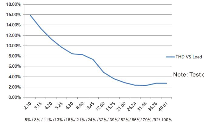
Note: Test data under 1050mA gear
