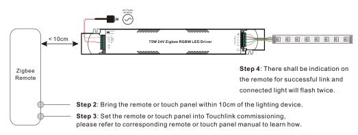
Note: 1) Directly TouchLink (both not added to a ZigBee network), each device can link with 1 remote.
