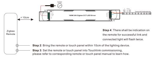
Note: 1) Directly TouchLink (both not added to a ZigBee network), each device can link with 1 remote. 2) TouchLink after both added to a ZigBee network, each device can link with max. 30 remotes.
