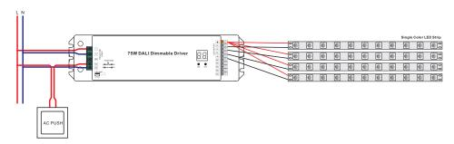
Note: all 4 channels are controlled together under this mode.
