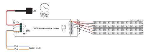
Note: The control gear will be discovered by DALI master as a DT6 device, 4 channels controlled together.
