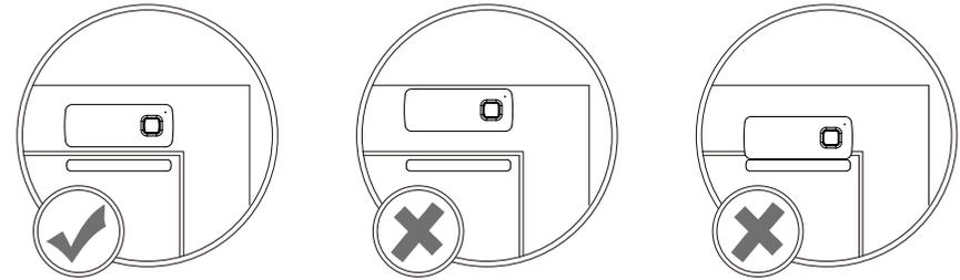
Correct positioning of the magnet in relation to the Sensor:
