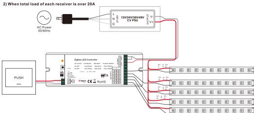
Note: please make sure the dial switches are at position for DIM mode as shown in above diagram.
