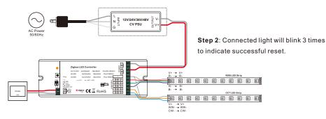
Note: All configuration parameters will be reset after the device is reset or removed from the network.
