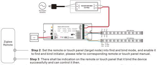
Note: Make sure the device and the remote or touch panel already added to the same Zigbee hub.
