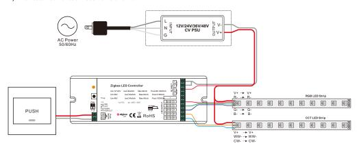
Note: please make sure the dial switches are at position for RGB+CCT mode as shown in above diagram.
