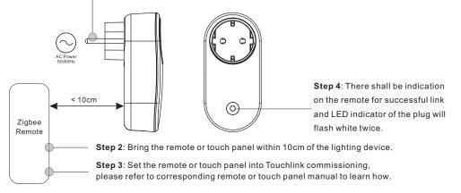
Note: 1) Directly TouchLink (both not added to a ZigBee network), each device can link with 1 remote.
