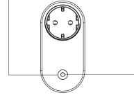
Step 4: LED indicator will flash white 6 times to indicate successful pairing. LED indicator will maintain the status before entering into network pairing mode if pairing fails.
