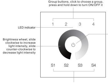
All ON/OFF button, click to switch ON/OFF all paired lighting devices Press and hold down to search and pair to ZigBee network or factory reset the dimmer switch.
