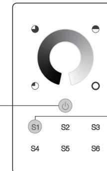
**Step 2:** From your zigbee controller or hub interface, choose to add device or accessory and enter Pairing mode as instructed by the controller.
