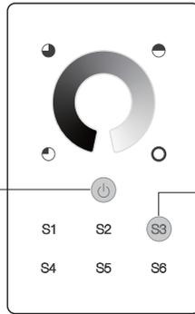
**Step 2:** Short press 5 times continuously to clear all bound lighting devices. LED indicator flashes 4 times for successful unbinding.
