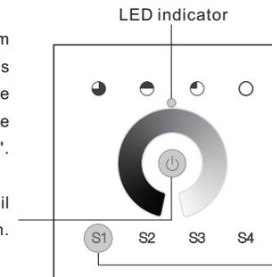
**Step 2:** From your zigbee controller or hub interface, choose to add device or accessory and enter Pairing mode as instructed by the controller.
