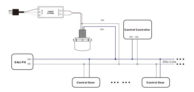
Note: please make sure the polarity of DALI signal of the sensor is correctly connected
