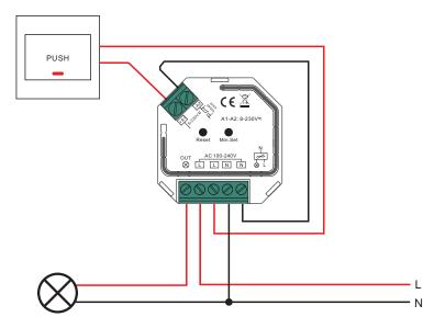
2) With Multiple Push Switches for Multiple Control Points
