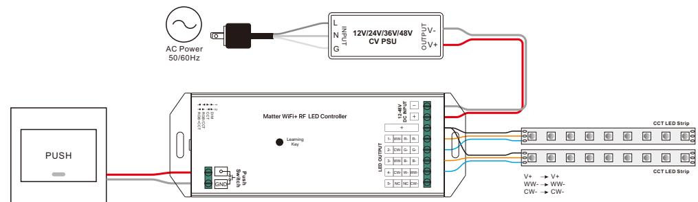
RGB/CCT mode / RGB+CCT mode: Work with RF remote
