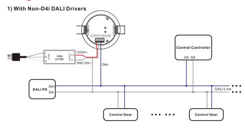
Note: please make sure the polarity of DALI of the sensor is correctly wired to the DALI PS.
