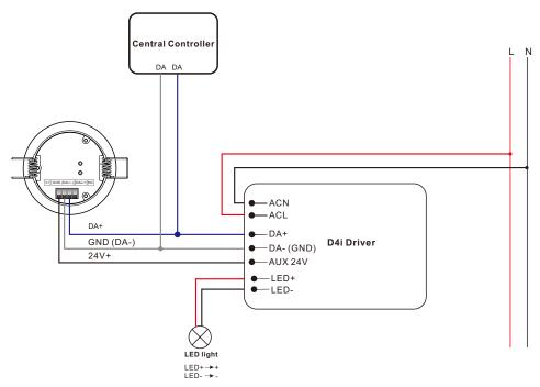
Note: please make sure the polarity of DALI of the sensor is correctly wired to the DALI PS.
