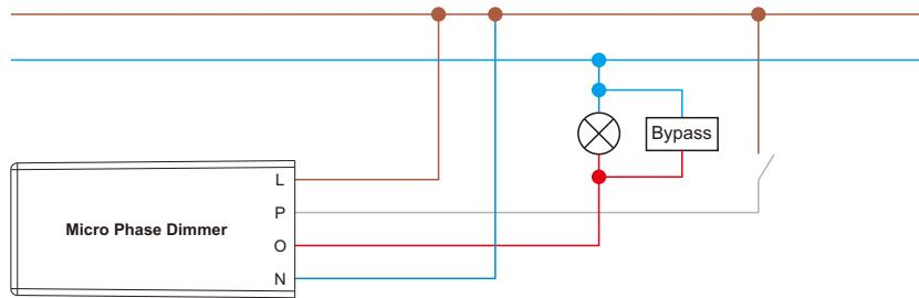
\* When using the device without neutral, the smart dimmer requires at least 20W @ 240 VAC of power consumption to operate. If the connected light has a smaller power consumption, then Bypass is needed for the device to work.
