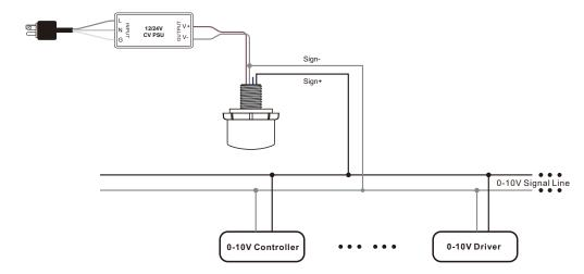
**Note:** please make sure the polarity of 0-10V signal of the sensor is correctly connected.
