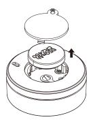
3. Replace the battery and reinstall the battery cover
