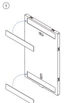
Method 1:Stick 3M glue on the back of the bracket and then stick the bracket to the wall
