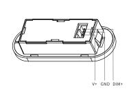
1 Reset Key: Press it to help withdraw the device from internet/APP, LED flashes quickly indicates success.
