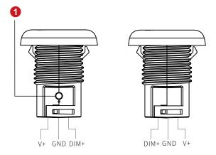
Reset Key: Press it to help withdraw the device from internet/APP, LED flashes quickly indicates success.
