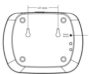
WiFi Reset switch: press and hold down for 10S then release, the blue WiFi indicator will go off and go on again, WiFi setting will be factory reset.
