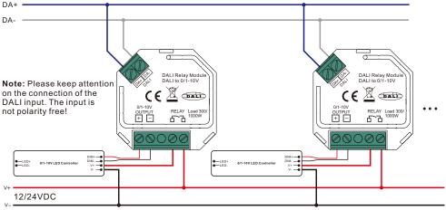
Note: the relay can also be connected to the input of the 12/24VDC PSU to switch 100-240V mains power.
