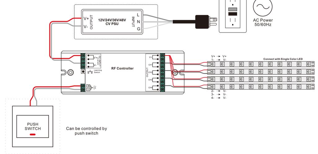
2) When total load of each receiver is over 20A
