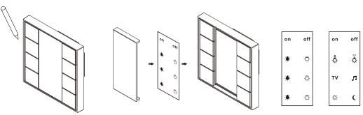
**Step 2:** Put the printed label into the central part.
