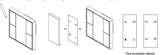
Step 1: Remove the white color central cover plate using a sharp tool such as
