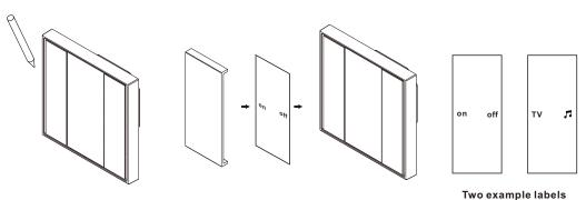
**Step 1:** Remove the white color central cover plate using a sharp tool such as tweezers.
