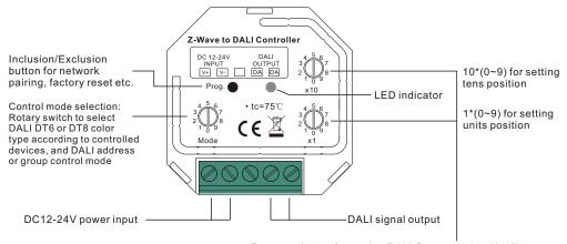
Rotary switches for setting DALI Group number (0-15) or Address number (0-63) to be controlled, the number equals to tens position plus units position
