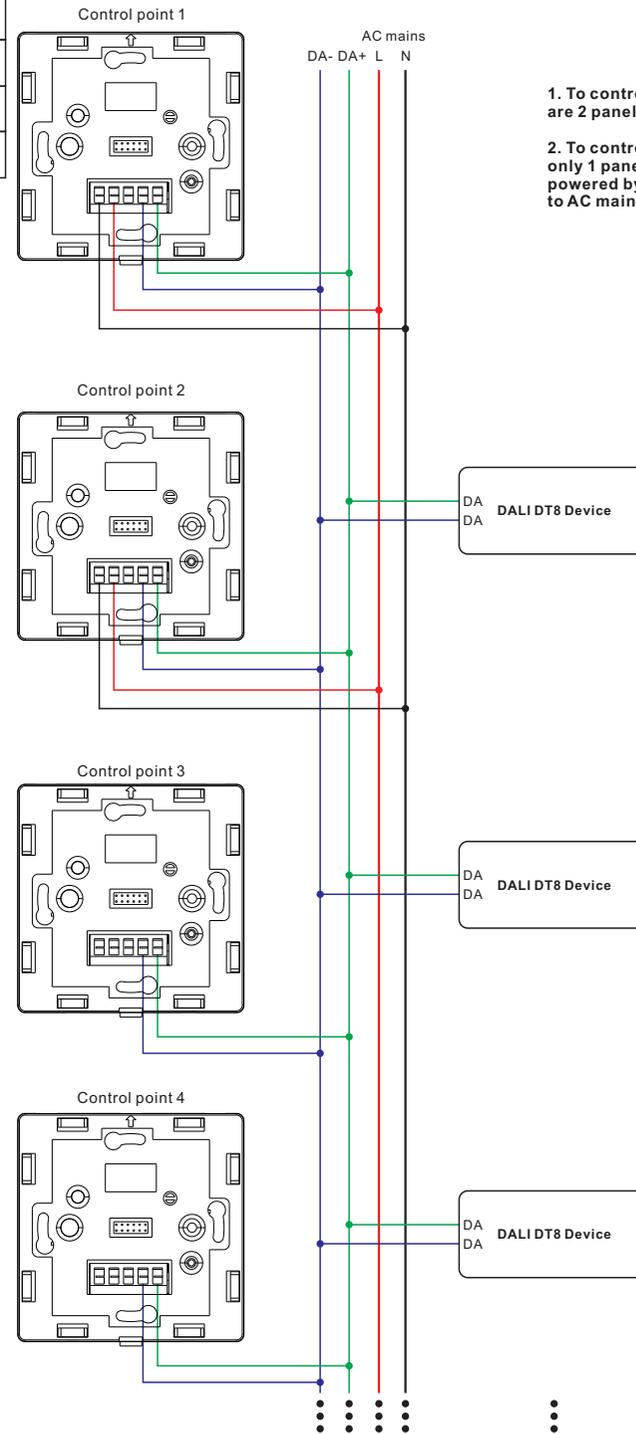
1. To control up to 100 ECG with the setup (Figure 2), there are 2 panels connected to AC mains.
