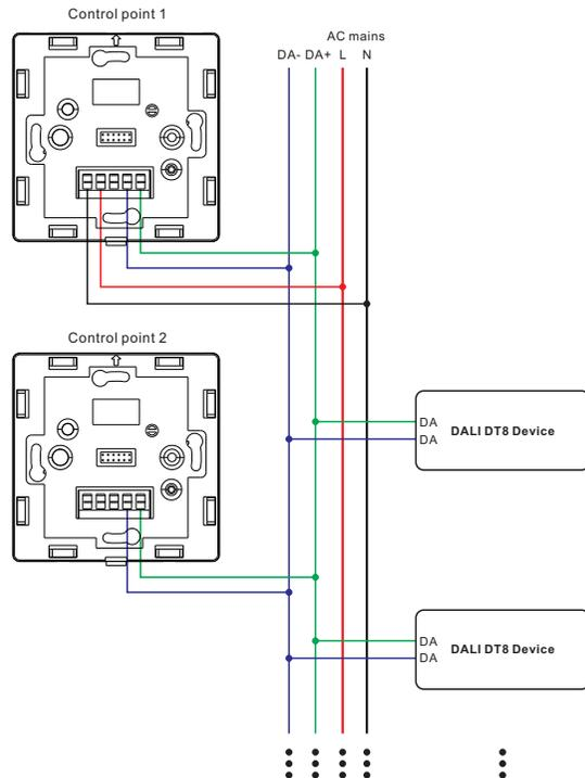
Figure 2: Wiring scheme with 2 DALI panels powered by AC mains to control up to 100 DALI ECG via broadcast or control 4 DALI groups.
