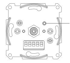
Remove the glass frame of the dimmer, the potentiometer will be visible, use a screwdriver to insert and rotate to adjust the dim off signal voltage
