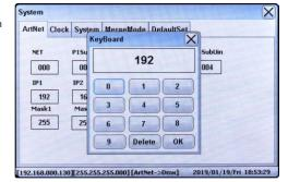
255.255.255 after set IP1-IP4 respectively. Once set, touch OK on the key board. Then close the System configuration window to confirm and save the setting.
