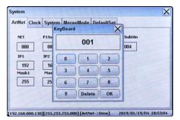
range is 1-255. Once set, touch OK on the key board. Then close the System configuration window to confirm and save the setting.
