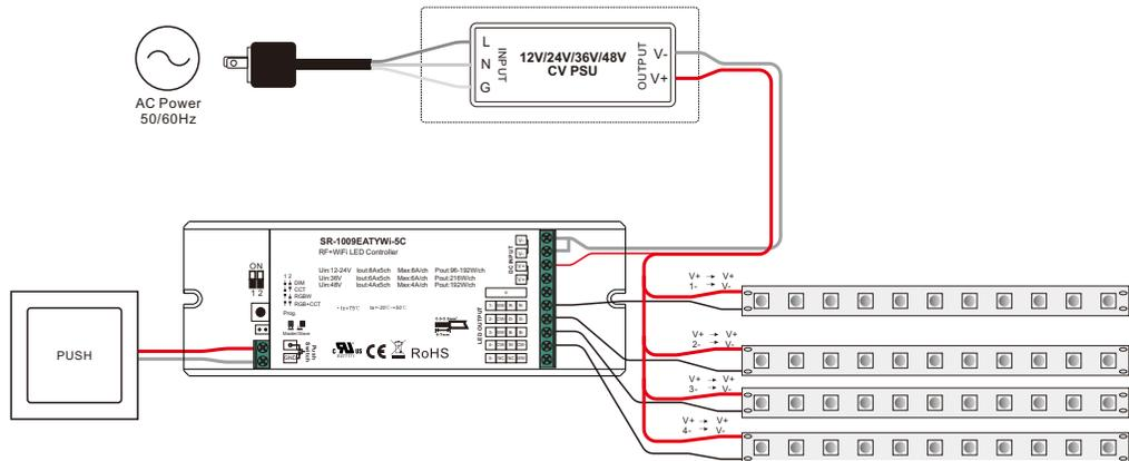
**Note:** please make sure the dial switches are at position for DIM mode as shown in above diagram.
