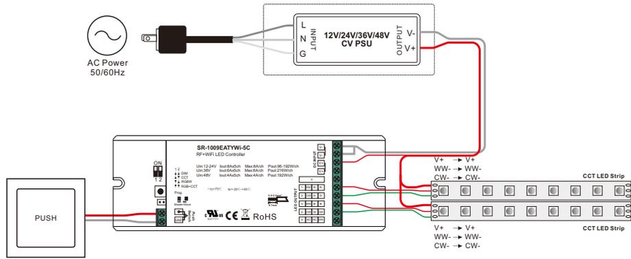
**Note:** please make sure the dial switches are at position for CCT mode as shown in above diagram.
