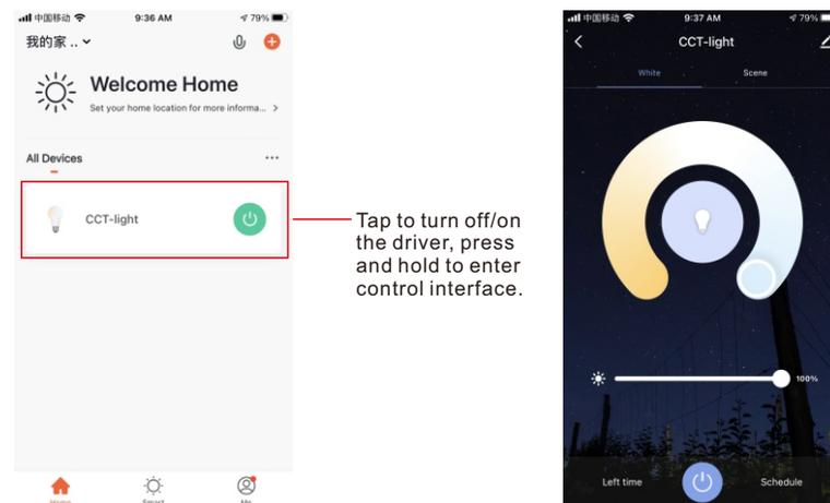
**Step 3:** Confirm that the driver is set to pairing mode and LED light blinks rapidly. Connecting starts, the WiFi LED controller will appear on the APP interface once added successfully.
