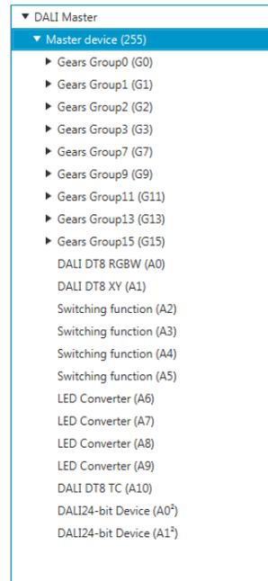
Click on "Done", the addressing guide window will be closed, meanwhile the device tree on the left of the main window will be loaded:
