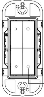
**Step 1:** Click the “Prog.” or “Reset” button on the light device 3 times continuously to set it into delete pairing to GP switch mode
