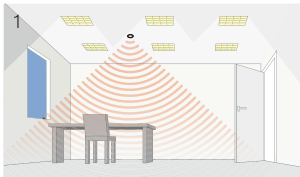
1. Power up the sensor. The load should come on immediately.
