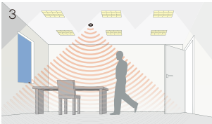
3. Enter the room or make some movement and check that the load switches on.
