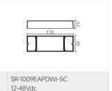
SR-1009EA Input Voltage 12-36Vdc **Output Current** 8A\*4CH Output Power 384-1152W Feature 8A/CH, CV
